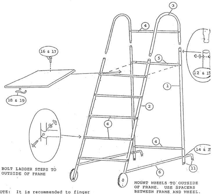
NOTE: It is recommended to finger tighten stand first. When completely assembled, tighten all nuts and bolts securely. Start with upper bolts on VERTICAL part #1 & #2 attaching to #3, Then bottom VERTICAL parts #1 & #2 attaching to part #6, proceed to tighten remaining HORITZONTAL part #4 & #5.
