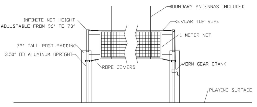
Posts Designed for 3.5" Existing Floor Sockets. First Team will provide socket adapters for other sized floor sockets at no charge upon request.
